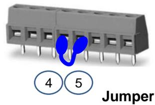
2) If there is a dual EOI, you should connect the wiring between #5 (external connector of the main EOI) and #5 (external connector of the dual EOI)
