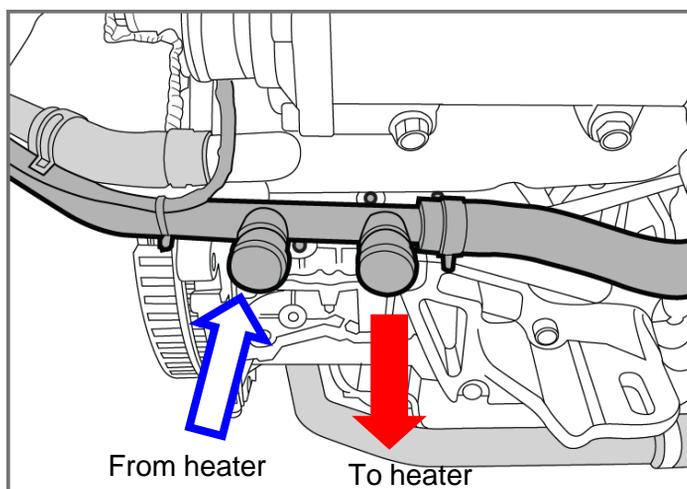
\* Outer diameter of pipe is  $\varnothing 17.3$  mm
