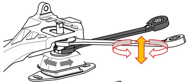
2) After alignment, place washer (③) on top of engine support bracket and tighten lock nut (④) while keeping the middle nut (②) from turning with a spanner.
